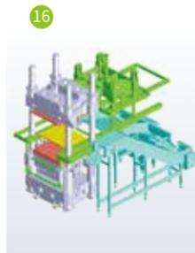
16 Auto ejecting device for bushing
