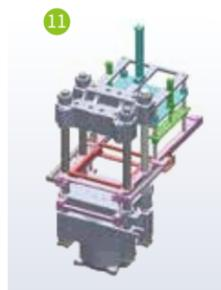
11 Downward ejecting device
