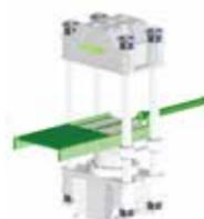
⑥ Lower mold sliding device
