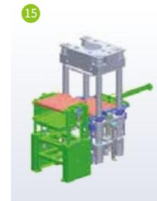
15 Double lower or middle mold exchange device (mold of big height)
