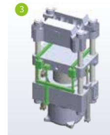
3 Bottom hydraulic mold separator
