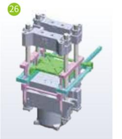
26 Ejecting device in clamping area
