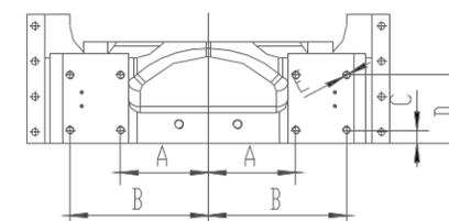
Robot Mounting Holes in the Fixed Platen
